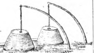
native Bellows for smelting Iron.
